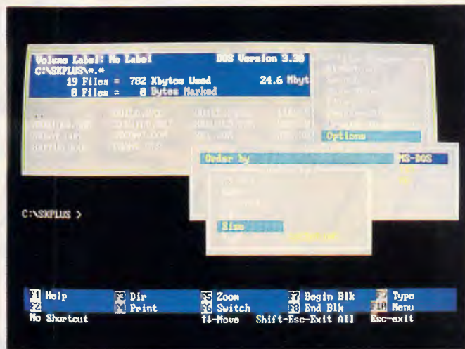
The SideKick Plus file manager allows directories to be sorted by filename, extension, size or date. It also supports File searches and disk formatting
