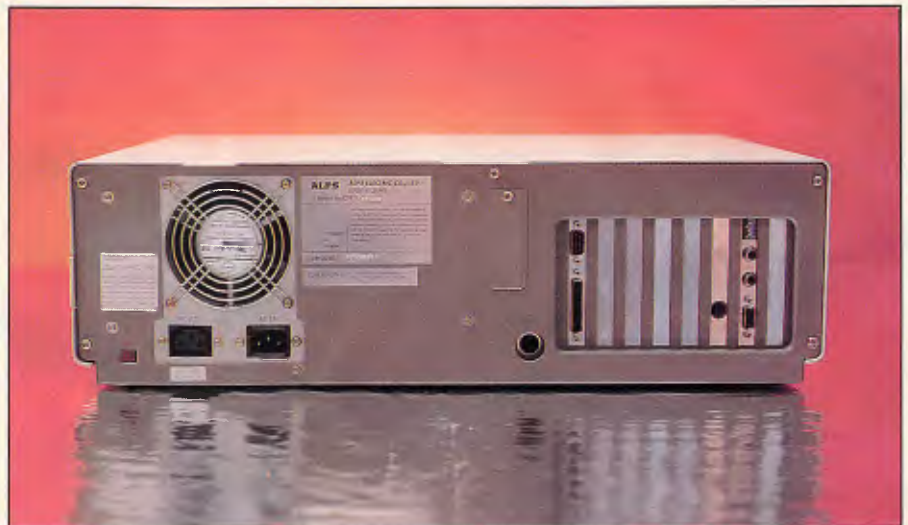
The rear of the NeoStar 386 reveals five free slots and VGA card outputs
