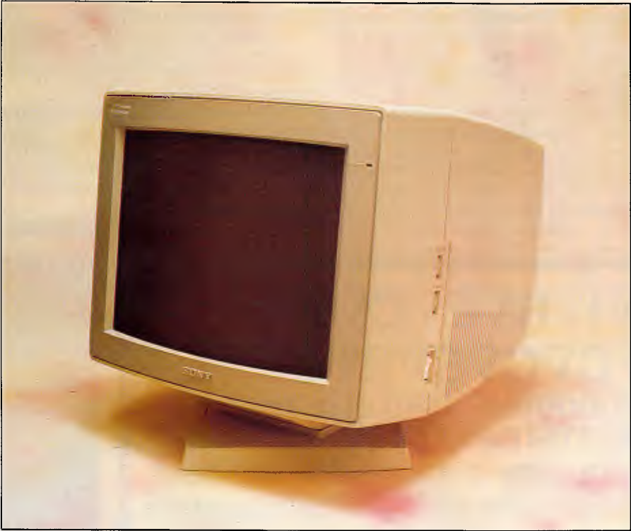
At 0.26mm, the Sony Multiscan CPD 1402E has the best shadowmask pitch
