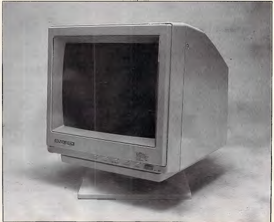
The second best shadowmask pitch is provided by the Eizo Flexscan 8060S, just 0.28mm
