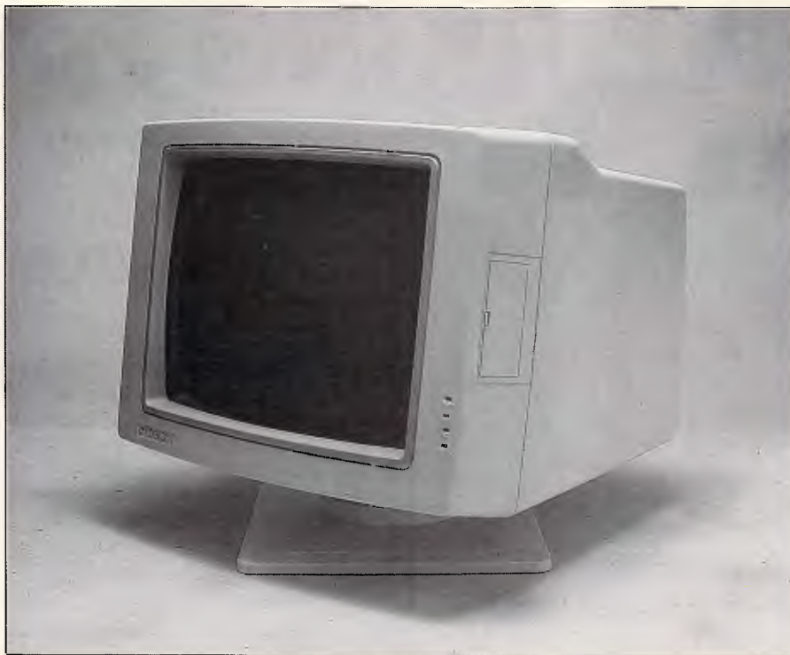
The Logitech Autosync TE5155 has its controls located behind a flip-open cover on the side
