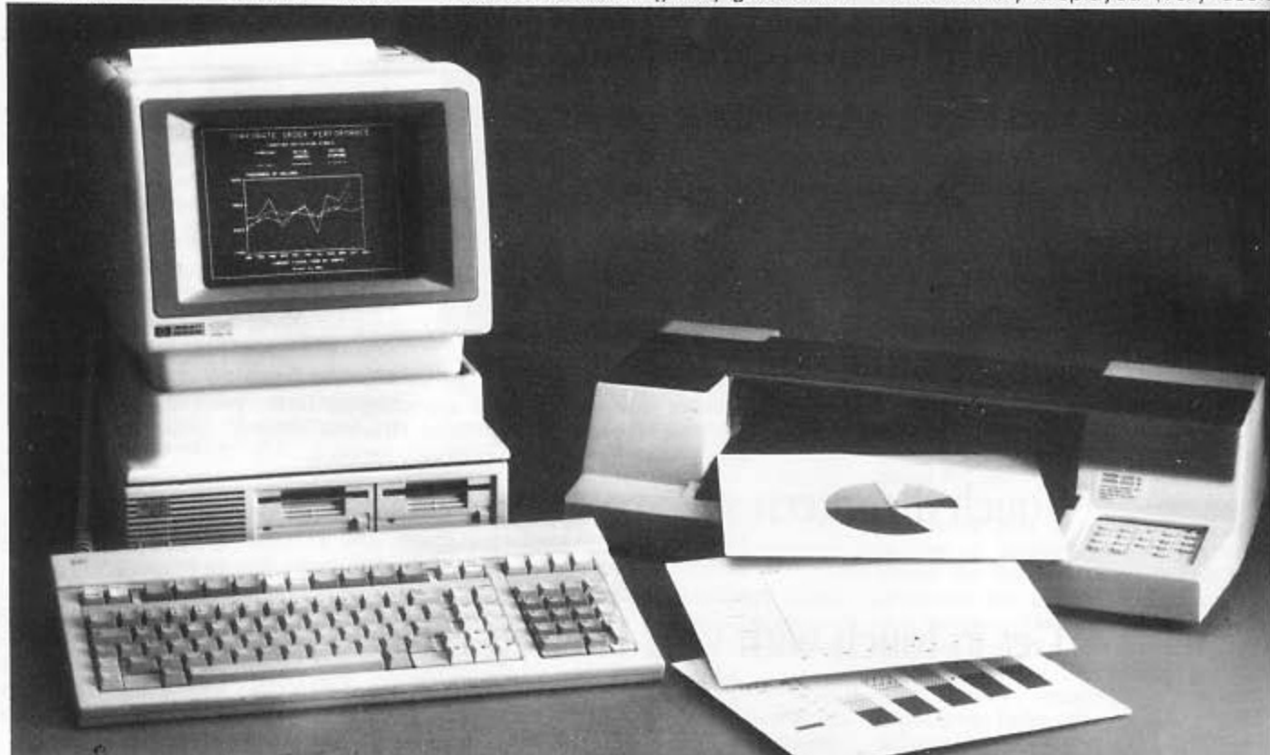
The HP 150 personal computer, with HPTouch, supports a full range of peripherals, including the new HP 7475 plotter.
