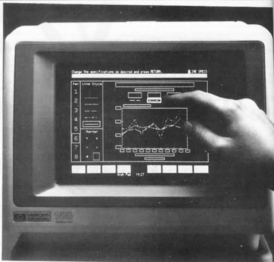
Touch makes applications programs like graphics easy to learn and use on the HP 150 personal computer.
