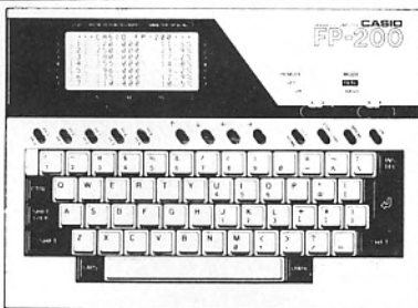
CASIO FP-200 Handy Personal Computer • 310(W) x 220(D) x 55.5(H) mm
