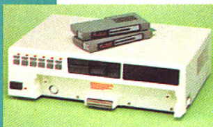
SV605 SUPER EXPANDER with disk drives and expansion cartridges
