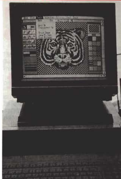
GEM Paint running on the Philips :Yes computer — one of the new range of applications packages using WIMPs (windows, icons, mouse and pull-down menus).
