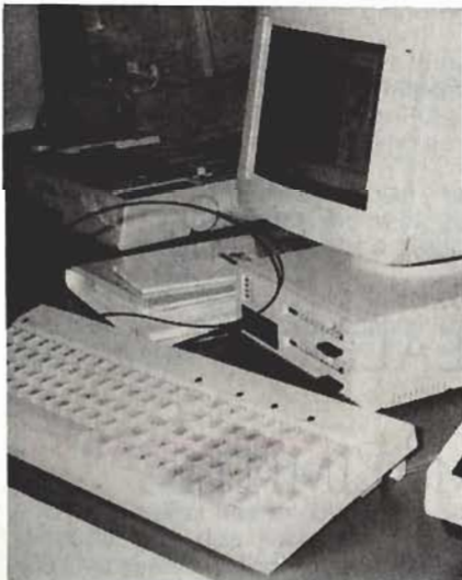
Apricot's new F2 model — 512 K of RAM, twin 720 K 3.5 inch disk drives, a mouse and GEM for £1495 (NZ$3750)
