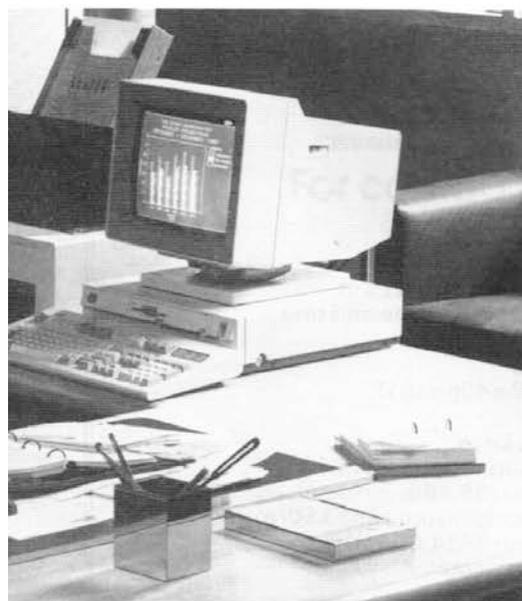
inch disk drives, a reduction in the number of expansion slots from eight to three, and the use of higher-density semiconductor packages. A secondary effect of these changes is a smaller power demand, which is satisfied with a 70-watt power supply.
