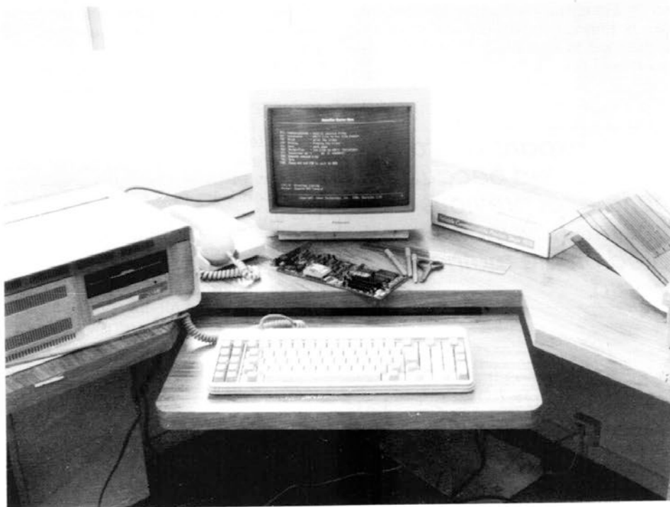
The addition of the Gammafax board (shown in front of the monitor) to a PC gives it the capability of the facsimile machine at right.
