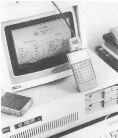
Figure 4: hand-held microcomputer connected to a PC
