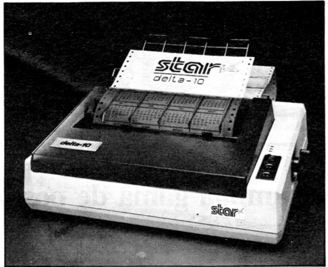
Delta 10 : 80 columnas, 160 cps. Delta 15 : 132 columnas, 160 cps.
