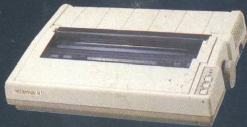
R 15 Compatible IBM PC, 8 K. buffer, NLO, 160 cps.
