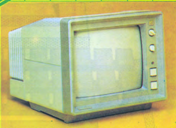
CT 900 SR 14" colour monitor PAL - CCIR with SOUND, RGB LINEAR- TTL COMPATIBLE
