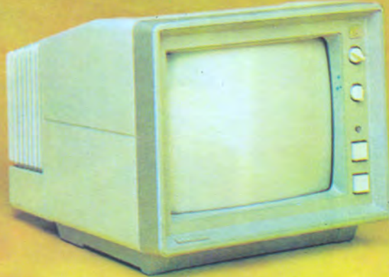
CT 900 SR 14" colour monitor PAL - CCIR with SOUND, RGB LINEAR- TTL COMPATIBLE
