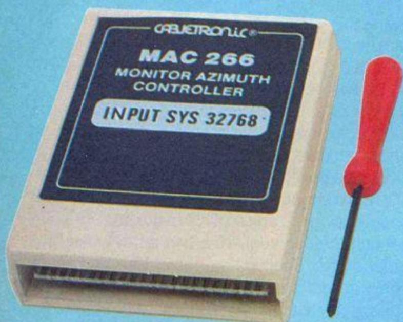
Cartridge monitor Azimuth controller for Commodore CBM 64/128. **ART. MAC 266.**
