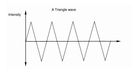
Each number represents the intensity of an individual section of the waveform. This is equivalent to the height of just one point in the above graph.
