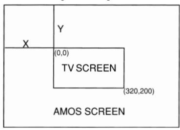
As you can see, the selected area of the screen is displayed through a view port positioned II at the coordinates *x* and *y*. You can move the view port through the whole screen by changing the values of these coordinates. This produces a smooth hardware scrolling effect which is perfect for many games. The size of your view port is taken from the dimensions you set in a previous call to the SCREEN DISPLAY command. II
