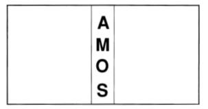
This sprite can be split into four horizontal segments each enclosing a single letter. The Amiga's hardware allows each section to be freely positioned anywhere on the current line, making a total of four *computed sprites*. Here's a diagram which illustrates this process.
