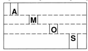
As you can see, a computed sprite is really just a small part of a hardware sprite displayed at a different horizontal screen position. Notice the line between each object. This is an unavoidable side effect of the repositioning process, and is generated by the Amiga's hardware.
