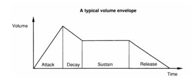
This sound is split up into four phases: Attack, decay, sustain and release.
