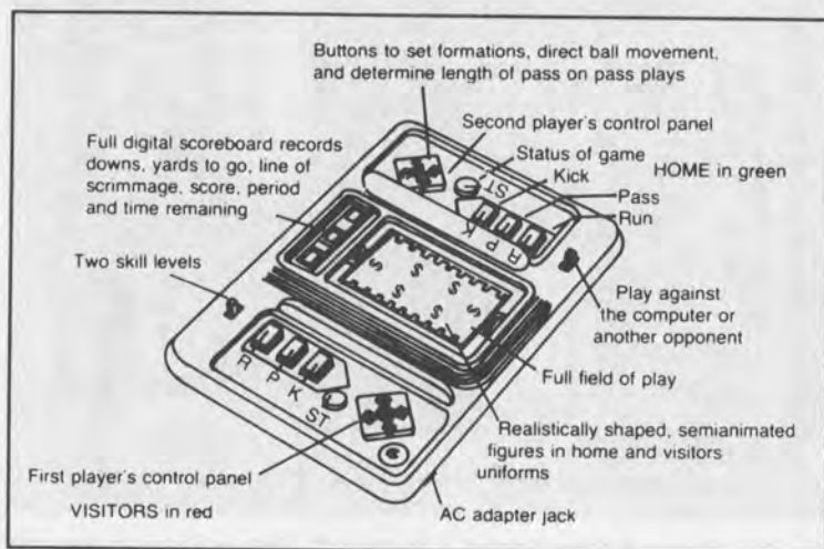
Fig. 9-5. Control functions for Electronic Color Football 4.
